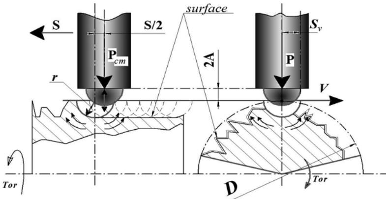
FIGURE 2. Plastic deformation by ultrasonic hardening treatment
